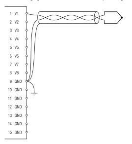
TMP01 device - for the sake of clarity only one thermocouple is shown. All pins are continuously protected against over-voltage of up to  $\pm 30$  V. The gold-plated connector pins ensure superior sensor connectivity. It is strongly recommended to use crimp D-sub connectors instead of a break-out board to ensure minimal cold-junction errors.
