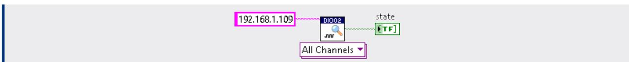
If only the logical state of one channel is to be read out, the device IP address or the DNS name and the channel number (from 1 to 8) are passed to instance *Single Channel*.
